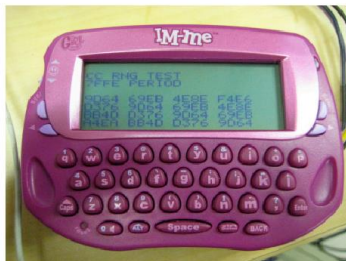
Figure 7: Girltech IMME, with modified firmware
